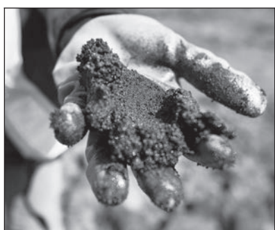
The oil in Canada's oil sands is bound up in dense, viscous soil that requires mining or deep steaming to free it.
